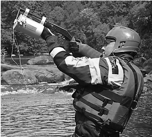
FIGURE 53. Bridger Line Gun, shown ready for deployment by instructor Michael McCarthy (Applied Rescue Technique, LLC). Image copyright Naval Company, Inc. Reprinted with permission.
