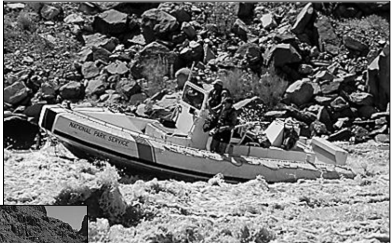
FIGURE 66. Canyonlands National Park jet boat in Cataract Canyon. A 450-hp diesel engine with a jet drive powers this 26-foot aluminum hulled vessel, which has a solid foam flotation collar.
