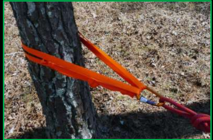
Basket Hitch Potential tri-axial loading issues
