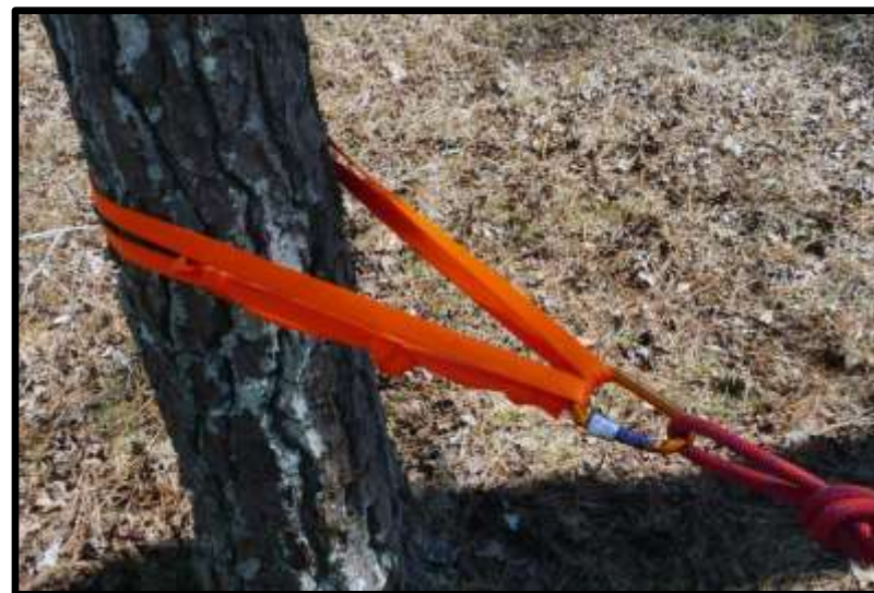
Basket Hitch Potential tri-axial loading issues
